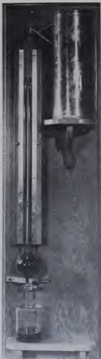
Figure 218.—Apparatus for direct measurement of surface moisture, absorption, and specific gravity of aggregate. PX-D-33523.
